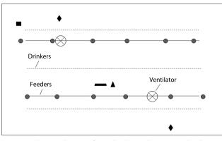
Figure 1. Schematic diagram of a poultry house showing sampling locations (■ Particulate Matter sampler (TEOM); — Andersen cascade impactor; ▲ Impingers; ● Gravitational plates; ◆ Temperature and relative humidity sensors)
